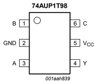
Fig. 2. Pin configuration SOT363-2 (TSSOP6)
