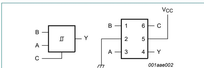
**Fig. 6. 2-input MUX**
