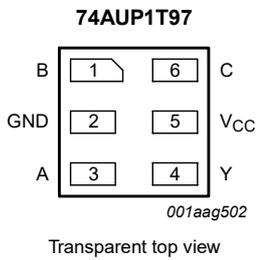
Fig. 4. Pin configuration SOT1115 and SOT1202 (XSON6)
