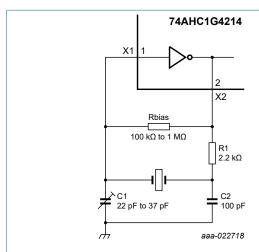
Fig. 8. External component connection for a crystal oscillator
