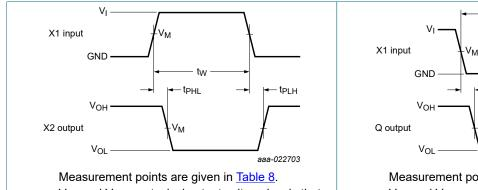
$V_{\text{OL}}$  and  $V_{\text{OH}}$  are typical output voltage levels that occur with the output load.
