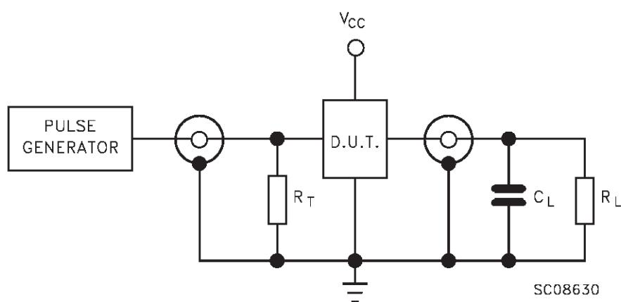
$C_L = 50 \text{ pF}$  or equivalent (includes jig and probe capacitance)
