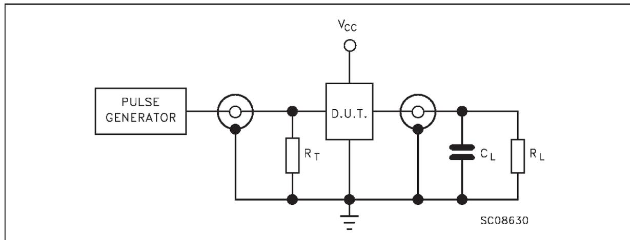
$C_L = 50$  pF or equivalent (includes jig and probe capacitance)
