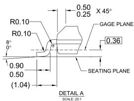
Figure 1. 14-Lead Small Outline Integrated Circuit (SOIC), JEDEC MS-012, 0.150" Narrow
