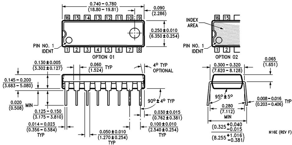
**16-Lead Molded Dual-In-Line Package (N)**
