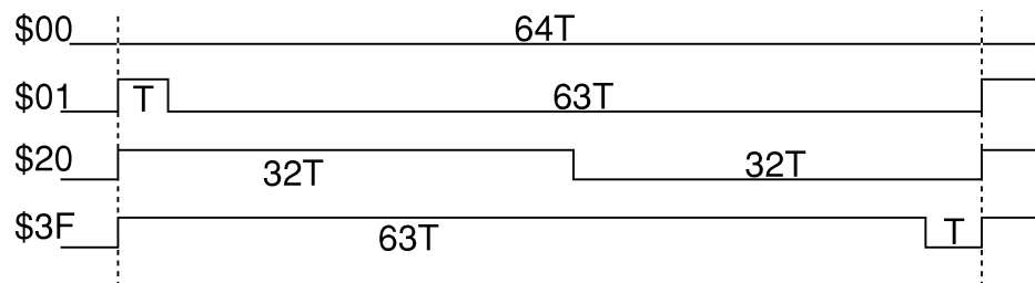
Figure 13-2. PWM Output Waveform Examples
