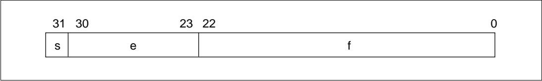
Figure 3.3 Floating-Point Number Format
