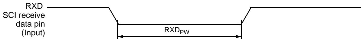
Figure 3-24 RXD Pulse Width
