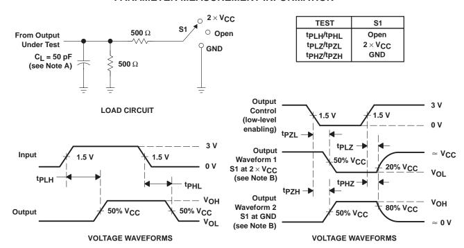
NOTES: A. C<sub>I</sub> includes probe and jig capacitance.
