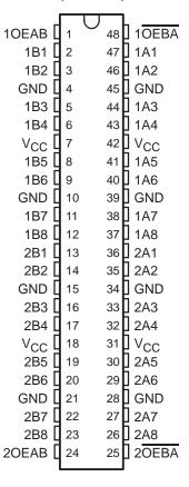
The dual-enable configuration gives the transceiver the capability to store data by simultaneously enabling OEAB and OEBA. Each output reinforces its input in this transceiver configuration. Thus, when both control inputs are enabled and all other data sources to the two sets of bus lines are at high impedance, the bus lines remain at their last states.
