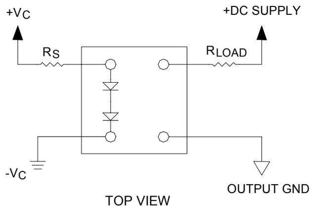
Figure 2. Terminal Connections
