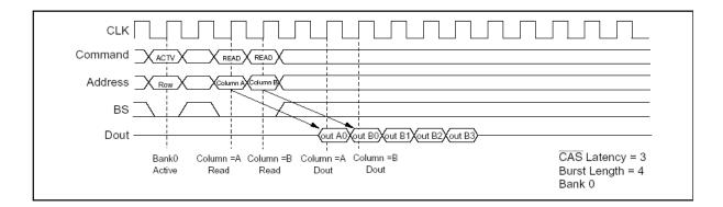
**2. Same bank, different ROW address:** When the ROW address changes on the same bank, consecutive read commands cannot be executed; it is necessary to separate the two read commands with a precharge command and a bank-active command.
