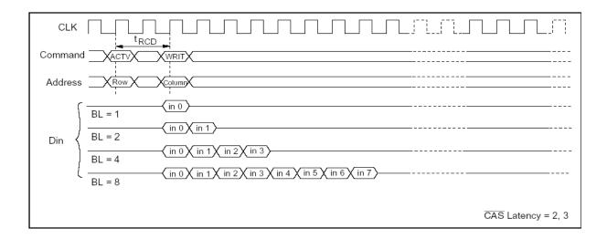
**2. Single write:** A single write operation is enabled by setting OPCODE (A9, A8) to (1, 0). In a single write operation, data is only written to the column address and the bank select address (BA0/BA1) specified by the write command set cycle without regard to the burst length setting. (The latency of data input is 0 clock.)
