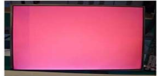
Vertical Block Source TAB IC Defect
