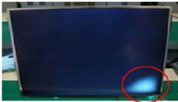
Panel Mura, Light leakage
