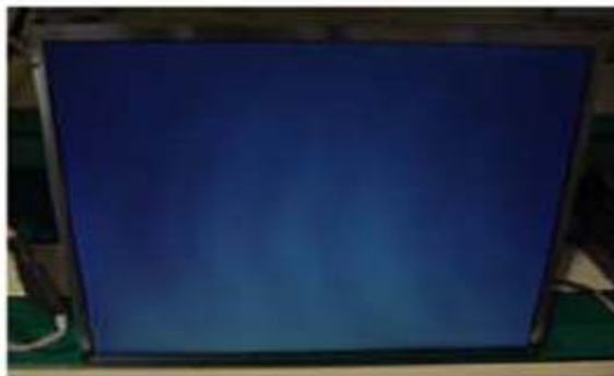
Panel Mura, Light leakage
