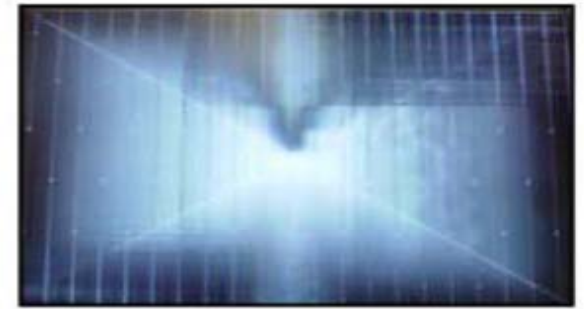
Solder defect, Short/Crack
