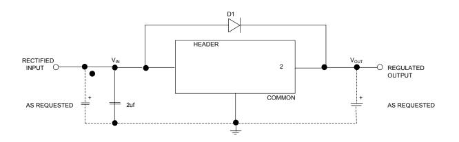
Note: D1 should be installed for input safety.
