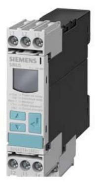
DIGITAL MONITORING RELAY FOR THREE-PHASE LINE VOLTAGE REVERSIBLE PHASE SEQUENCE PHASE FAILURE 3X 160 TO 690V AC 50 TO 60 HZ UNDERVOLT. AND OVERVOLT. 160-690V HYSTERESIS 1-20V 0-20S EACH FOR UMIN AND UMAX 1 W FOR UMIN 1W FOR UMAX SCREW TERMINAL REPLACEMENT PRODUCT F. 3UG3041-1BP50
