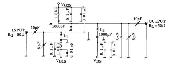
L<sub>1</sub>: 1 mm Ag plated copper wire, 2 turns, 8 mm ID
