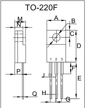
PIN 1. PIN 2. PIN 3. BASE COLLECTOR EMITTER
