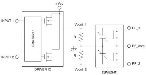
Note: 1. Operate the driving voltage with the high-side switch (Vcont\_1 & Vcont\_2, not ground).
