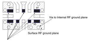
Connect **ALL** RF ground pads to the surface RF ground plane directly.
