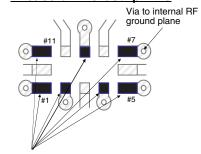
Connect **EACH** RF ground pad to the internal RF ground plane through the via placed to the RF ground pad.
