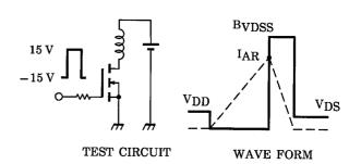
$$\begin{aligned} &RG = 25~\Omega \\ &V_{DD} = 90~V,~L = 4.76~mH \end{aligned} \qquad E_{AS} = \frac{1}{2} \cdot L \cdot I^2 \cdot \left( \frac{B_{VDSS}}{B_{VDSS} - V_{DD}} \right)$$
