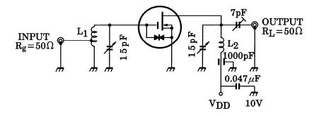
$L_1{:}~1.0~mm\varphi$  silver plated copper wire 4.0 T, 8 mm $\varphi$  ID TAP at 1.0 T from coil end
