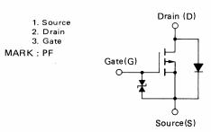
(Diode in the figure is the parasitic diode.)
