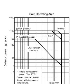
Collector-emitter voltage  $V_{CE}$  (V)
