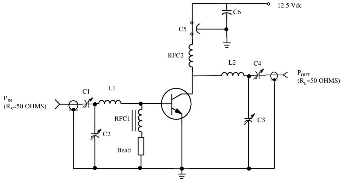
**Figure 1 - 175 MHz RF AMPLIFIER CIRCUIT FOR G<sub>PE</sub>,
