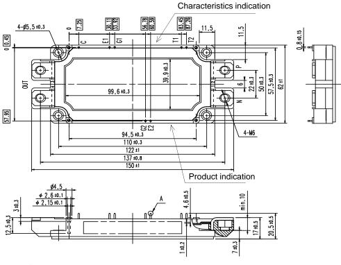
NOTE) \_\_\_\_\_ shows theoretical dimension and tolerance is </u> ቀ 💋.5
