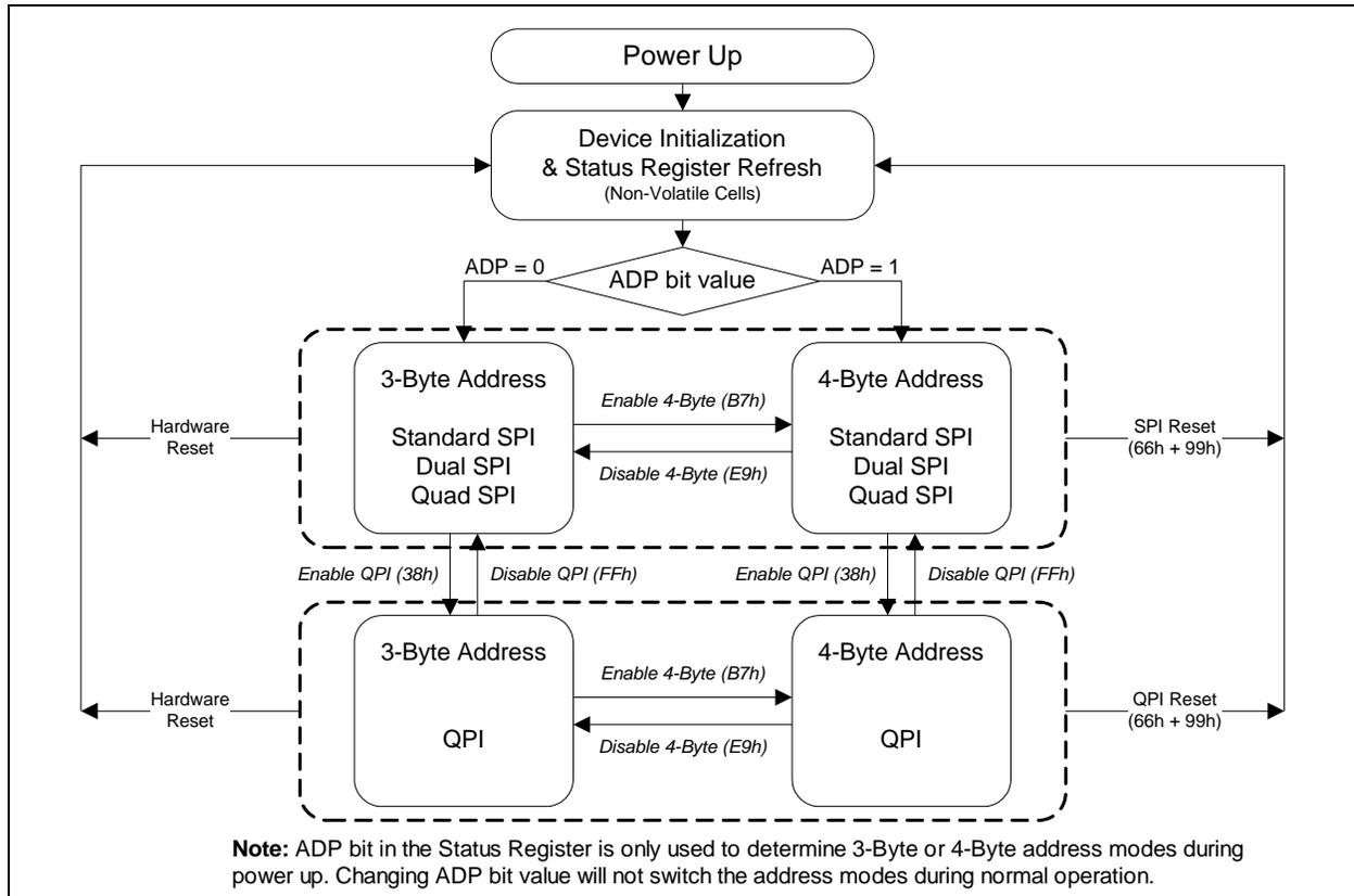
Figure 3. W25Q01JV Serial Flash Memory Operation Diagram
