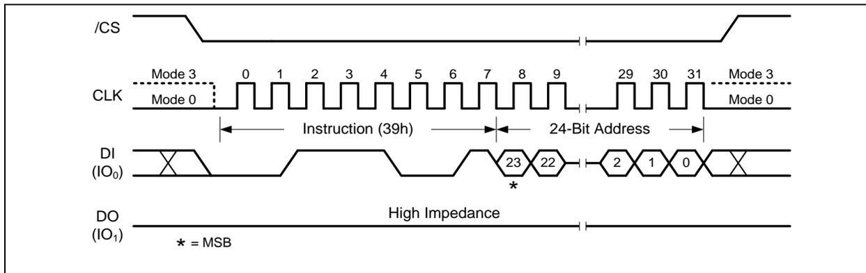
Figure 60a. Individual Block Unlock Instruction (SPI Mode)
