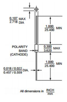
Lead Material: copper clad steel Lead Finish: tin/lead Marking: part number and cathode band Weight: 0.2 grams Polarity: diode to be operated with the cathode band end negative Mounting Position: any
