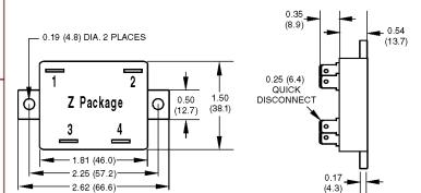
NOTE: All dimensions are nominal. We do not recommend mounting the terminal side of the SSR to a flat PCB (printed circuit board) or other flat surface, because there may be some variation in terminal height or alignment from one terminal to another and from one SSR to another.
