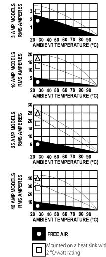
Mounted on a heat sink with
