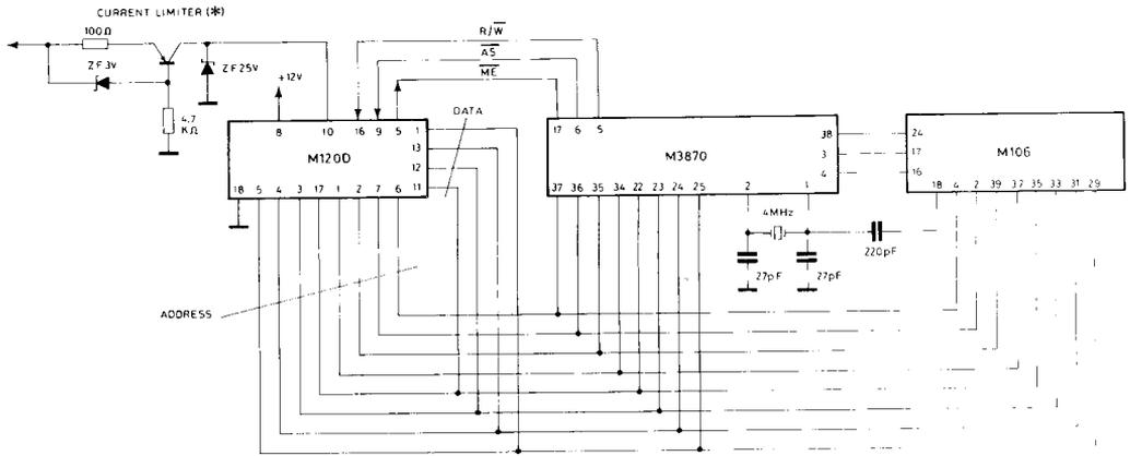
(\*) This circuit is necessary when  $V_{pp}$  maximum rating can be exceeded, even if for short periods as voltage spikes.
