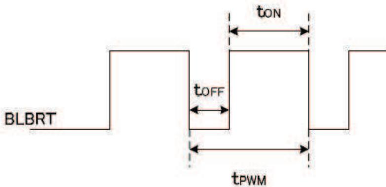
$t_{ON}, t_{OFF} \geq 50 \mu s.$
