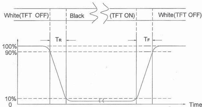
Note (4): This shall be measured at center of the screen.
