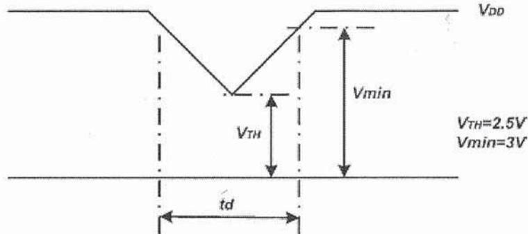
If  $V_{TH} < V_{DD} \leq V_{min}$ , then  $t_d \leq 10ms$ ; When the voltage return to normal our panel must revive automatically.
