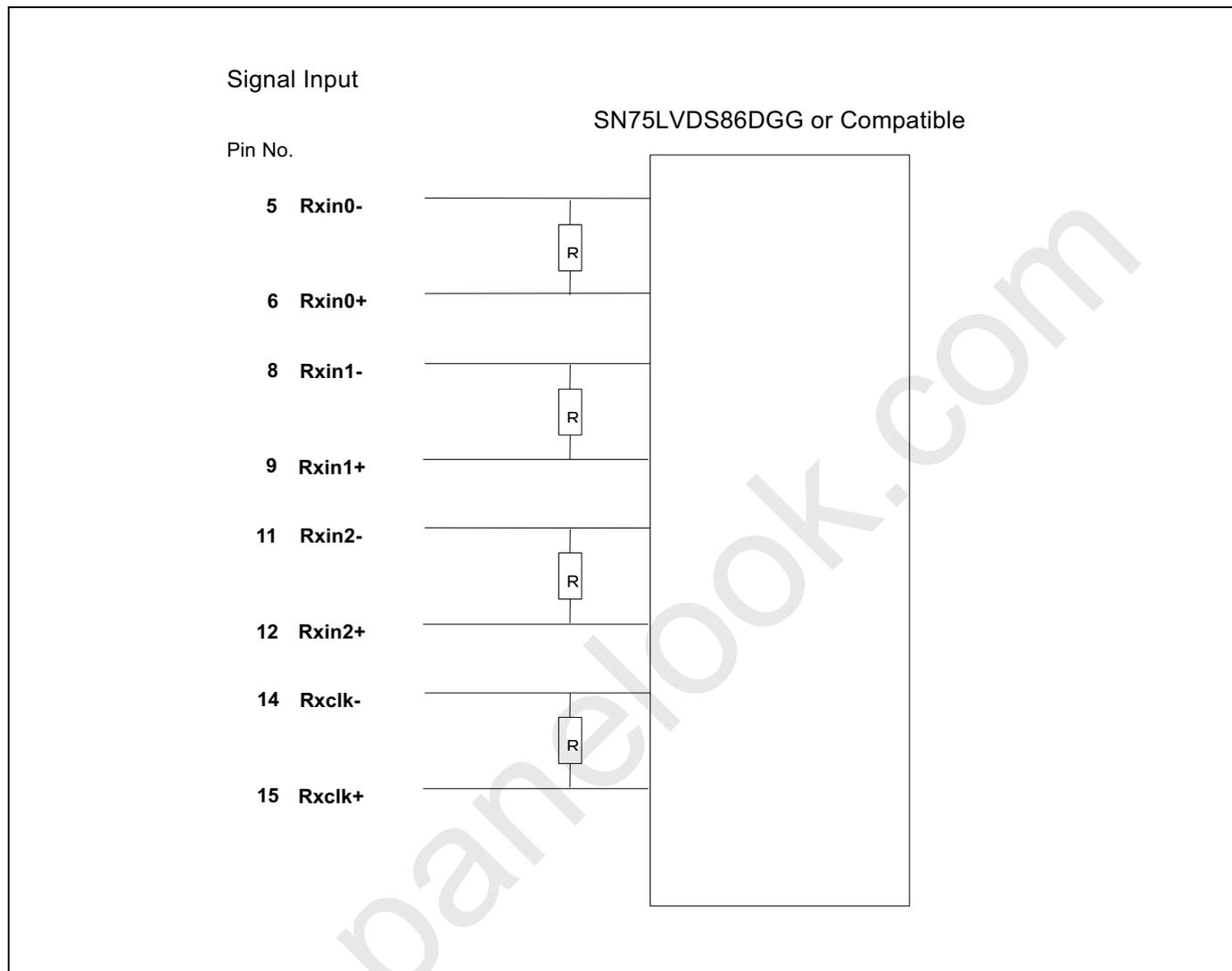
The module uses a 100 ohm resistor between positive and negative data lines of each receiver input.
