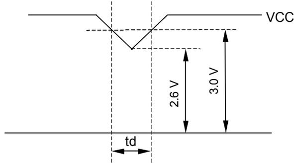
\*2)  $\text{VCC} = +3.3\text{ V}$ ,  $f_H = 48.4\text{ kHz}$ ,  $f_V = 60\text{ Hz}$ ,  $f_{\text{CLK}} = 65\text{ MHz}$
