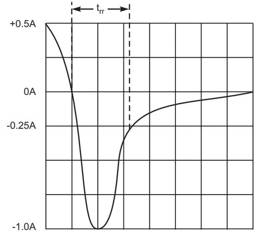
Fig. 5 Reverse Recovery Time Characteristic and Test Circuit
