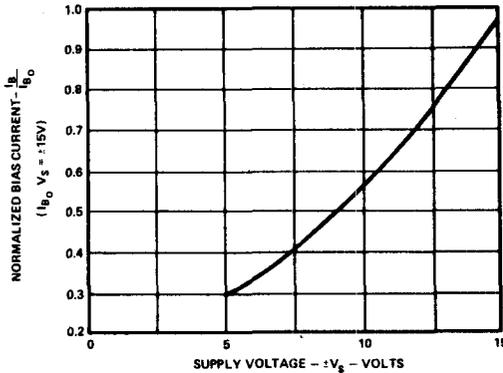
Figure 1. Normalized Bias Current vs Supply Voltage
