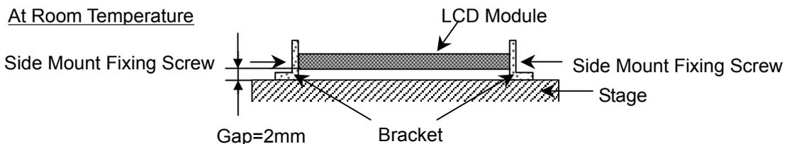
Note (5) At testing Vibration and Shock, the fixture in holding the module has to be hard and rigid enough so that the module would not be twisted or bent by the fixture.
