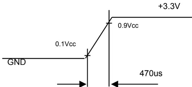
Note (3) The specified power supply current is under the conditions at  $V_{CC} = 3.3\text{ V}$ ,  $T_a = 25 \pm 2\text{ }^\circ\text{C}$ , DC Current and  $f_v = 60\text{ Hz}$ , whereas a power dissipation check pattern below is displayed.
