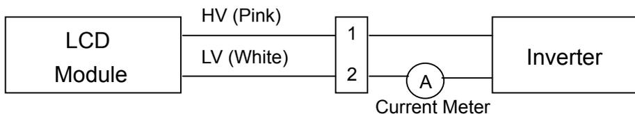
Note (2) The voltage shown above should be applied to the lamp for more than 1 second after startup. Otherwise the lamp may not be turned on.
