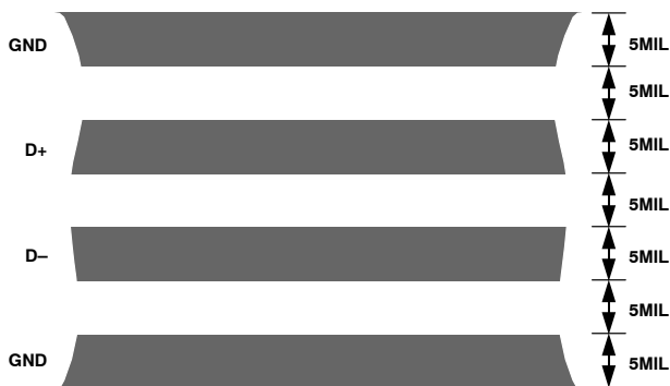
Figure 16. Typical Arrangement of Signal Tracks
