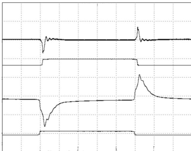
Figure 15: Output voltage response to step-change in load current lout2 and lout1 (75%-50%-75% of I_o , max; di/dt = 2.5A/\mu s ). Load cap: 470 \mu F , 35m \Omega ESR solid electrolytic capacitor and 1 \mu F ceramic capacitor. Ch1=Vout1 (50mV/div), Ch2=lout1 (10A/div), Ch3=Vout2 (100mV/div), Ch4=lout2 (10A/div) Scope measurement should be made using a BNC cable (length shorter than 20 inches). Position the load between 51 mm to 76 mm (2 inches to 3 inches) from the module.
