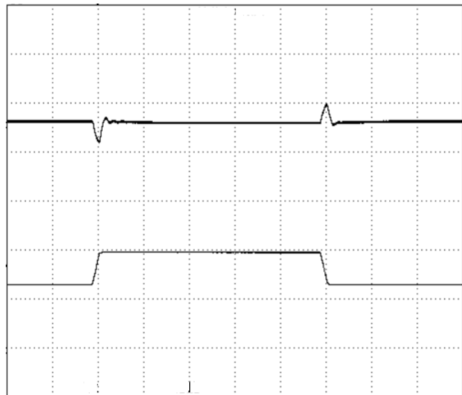
Figure 11: Output voltage response to step-change in load current lout1 (75%-50%-75% of I_o , max; di/dt = 0.1A/\mu s ) at lout2=0. Load cap: 10\mu F , tantalum capacitor and 1\mu F ceramic capacitor. Ch1=Vout1 (50mV/div), Ch2=lout1 (5A/div), Scope measurement should be made using a BNC cable (length shorter than 20 inches). Position the load between 51 mm to 76 mm (2 inches to 3 inches) from the module.
