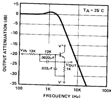
FIGURE 4: Frequency Attenuation Characteristics of the Output Buffer
