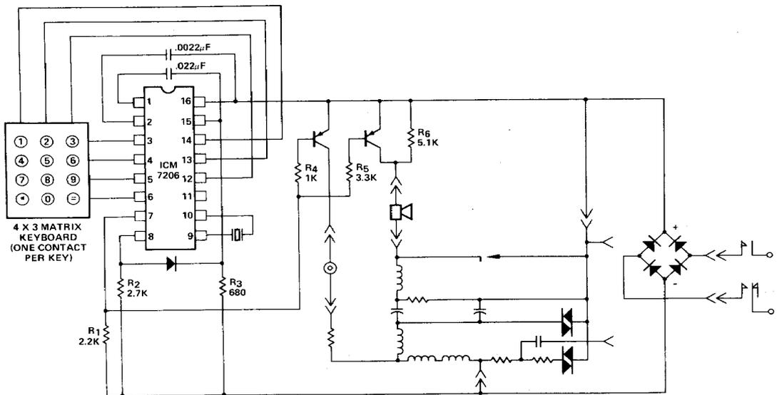
**NOTE:** If dual contact keyboard is used, common should be left floating.
