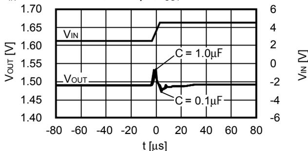
$V_{IN} = 4.5\text{ V} \rightarrow 2.5\text{ V}$ ,  $t_r = 5\ \mu\text{s}$ ,  $I_{OUT} = 100\text{ mA}$
