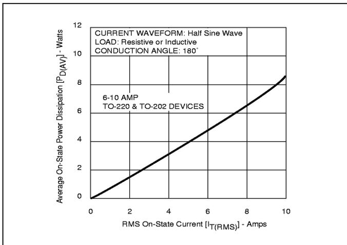
Figure 5.17 Power Dissipation (Typical) vs RMS On-State Current
