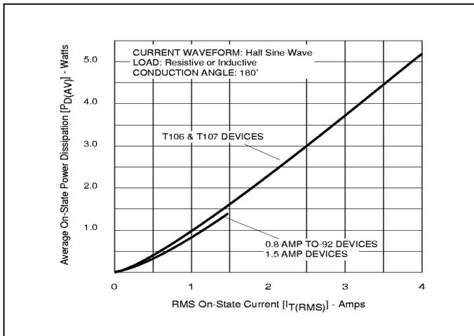
Figure 5.16 Power Dissipation (Typical) vs RMS On-State Current
