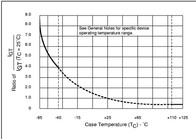
Figure 5.10 Normalized DC Gate-Trigger Current vs Case Temperature
