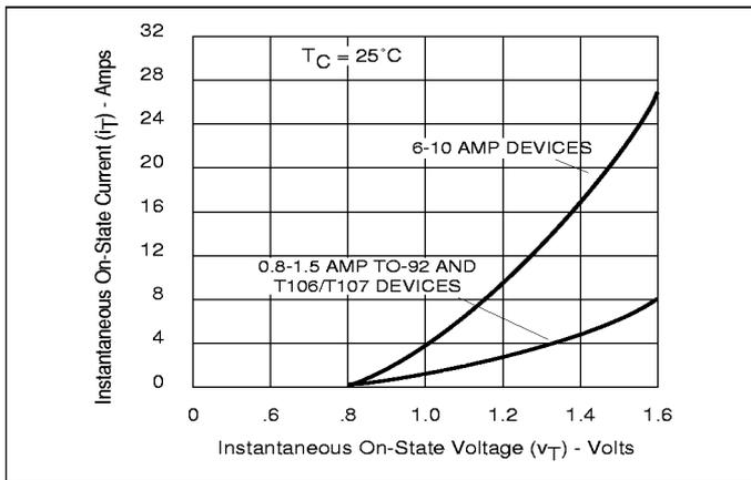
Figure 5.11 Instantaneous On-State Current vs On-State Voltage (Typical)
