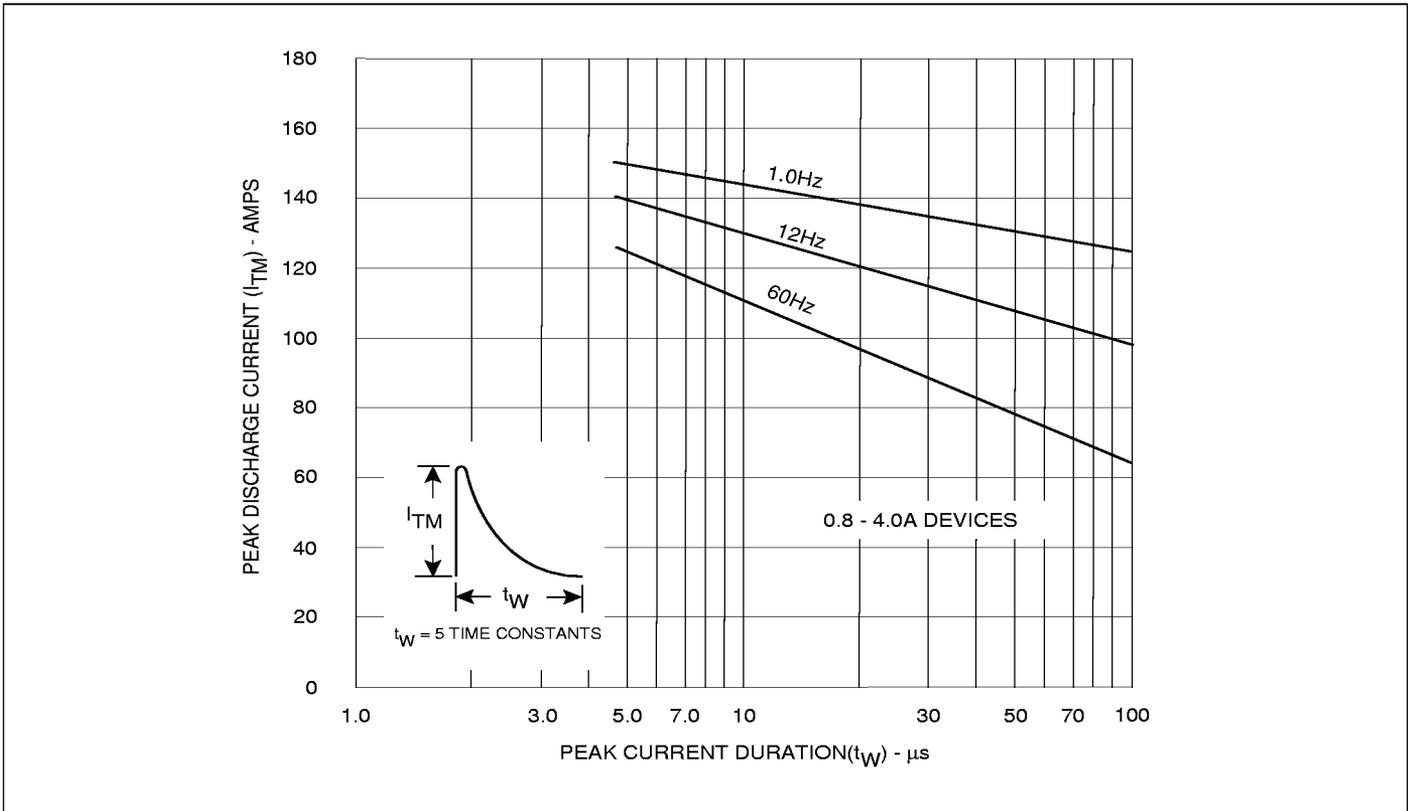
Figure 5.20 Peak Repetitive Capacitor Discharge Current
