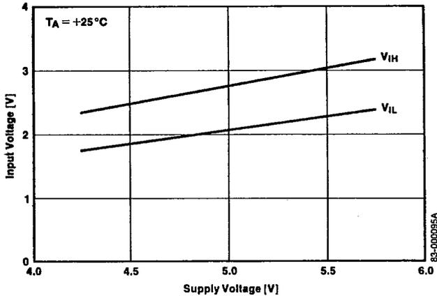
**Input Voltage vs Supply Voltage
