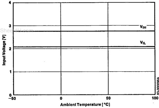
**Input Voltage vs Ambient Temperature
