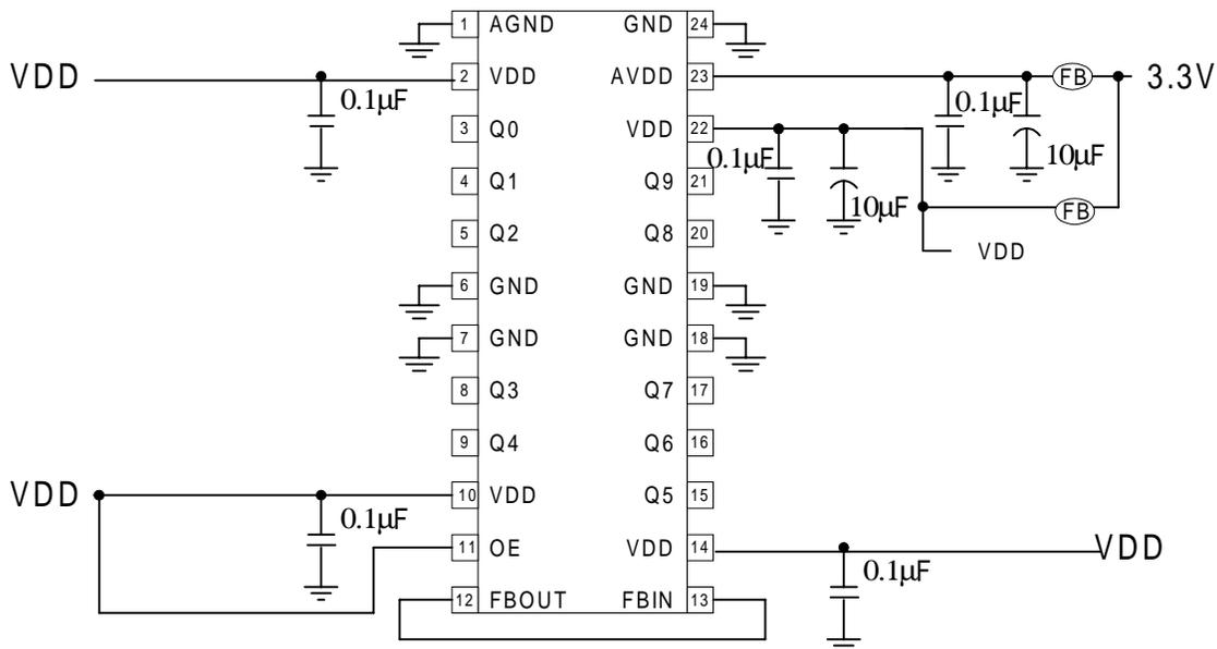
**Figure 1. Schematic**
