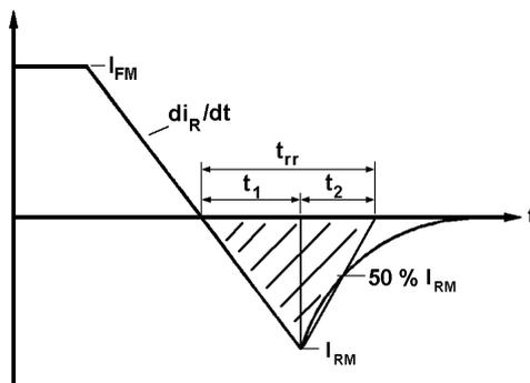
(ii) Q<sub>rr</sub> is based on a 150μs integration time.
