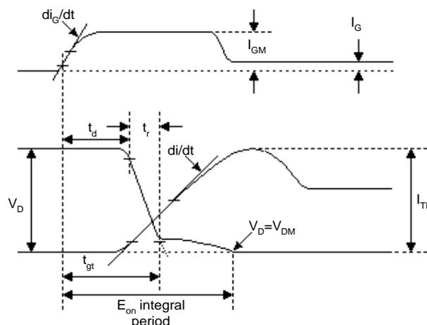
Diagram 9, Turn-on wave-diagrams.
