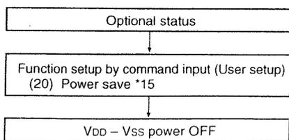
Set the time (t<sub>L</sub>) from power save to turning off the V<sub>DD</sub> - V<sub>SS</sub> power (V<sub>DD</sub> - V<sub>SS</sub> = 1.8 V) longer than the time (t<sub>H</sub>) when the potential of V<sub>5</sub> ~ V<sub>1</sub> becomes below the threshold voltage (approximately 1V) of the LCD panel.
