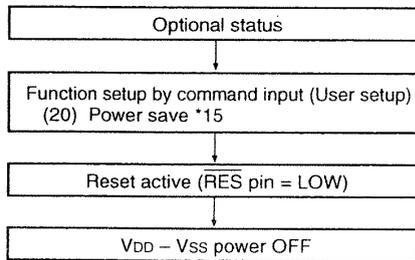
Set the time (t<sub>L</sub>) from reset active to turning off the V<sub>DD</sub> - V<sub>SS</sub> power (V<sub>DD</sub> - V<sub>SS</sub> = 1.8 V) longer than the time (t<sub>H</sub>) when the potential of V<sub>5</sub> ~ V<sub>1</sub> becomes below the threshold voltage (approximately 1 V) of the LCD panel. For t<sub>H</sub>, refer to the <Reference Data> of this event. When t<sub>H</sub> is too long, insert a resistor between V<sub>5</sub> and V<sub>DD</sub> to reduce it.
