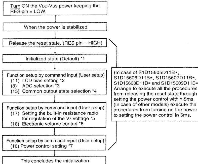
② When the built-in power is not being used immediately after turning on the power:
