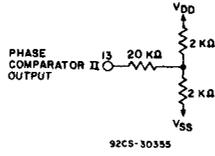
Fig. 11 - Phase comparator II output loading circuit.
