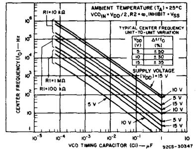
Fig. 4 - Typical center frequency as a function of C<sub>1</sub> and R<sub>1</sub> at V<sub>DD</sub> = 5 V, 10 V, and 15 V.
