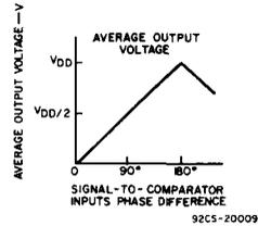
Fig. 2 — Phase-comparator I characteristics at low-pass filter output.
