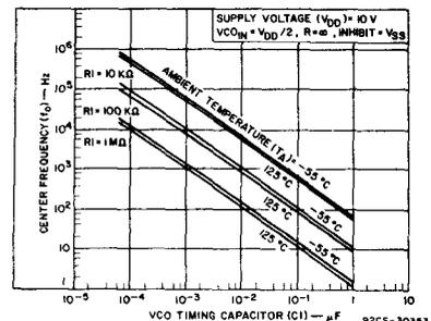
Fig. 5 - Center frequency as a function of C<sub>1</sub> and R<sub>1</sub> for ambient temperatures of -55°C to 125°C.
